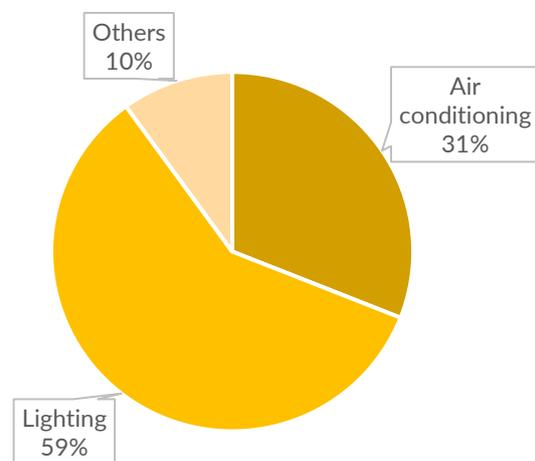
Figure 6: Commercial building electricity consumption breakdown<sup>13</sup>
