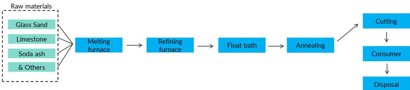
Figure 21: Schematic diagram of supply chain of glass industry
