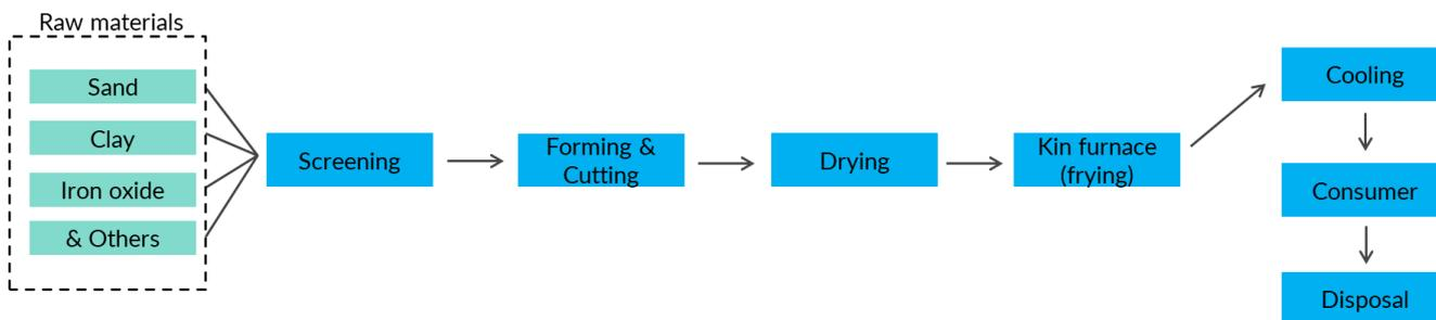
Figure 22: Schematic diagram of supply chain of brick industry
