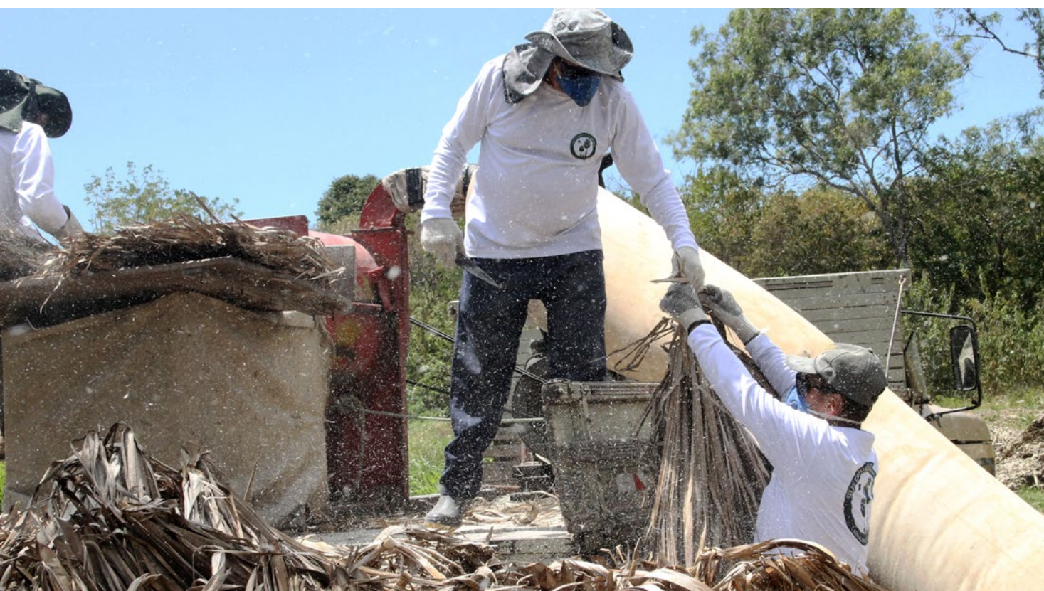
Image 43: Powder loss in the beating process. Source: Caatinga Association Collection.
